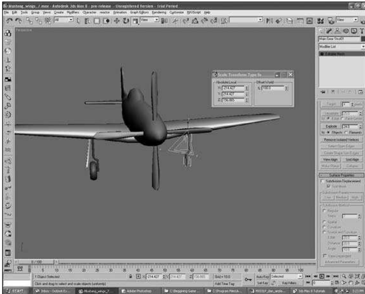
Figure 4.58 Scale the main strut in the negative X.
