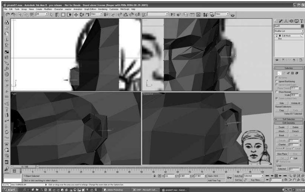
Figure 6.77 Weld some of the vertices from the extrusion.
