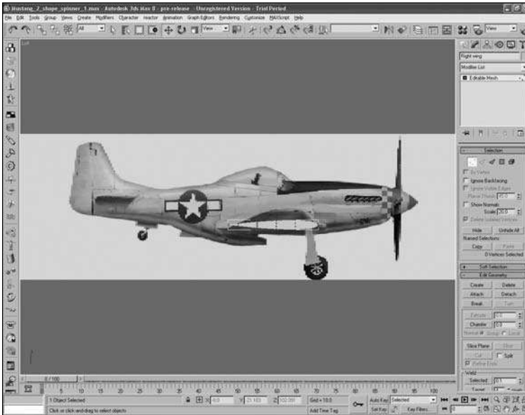
Figure 4.37 Shape the box into a symmetrical wing.
