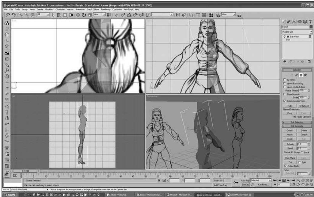
Figure 6.62 Select the mirror seam polygons.
